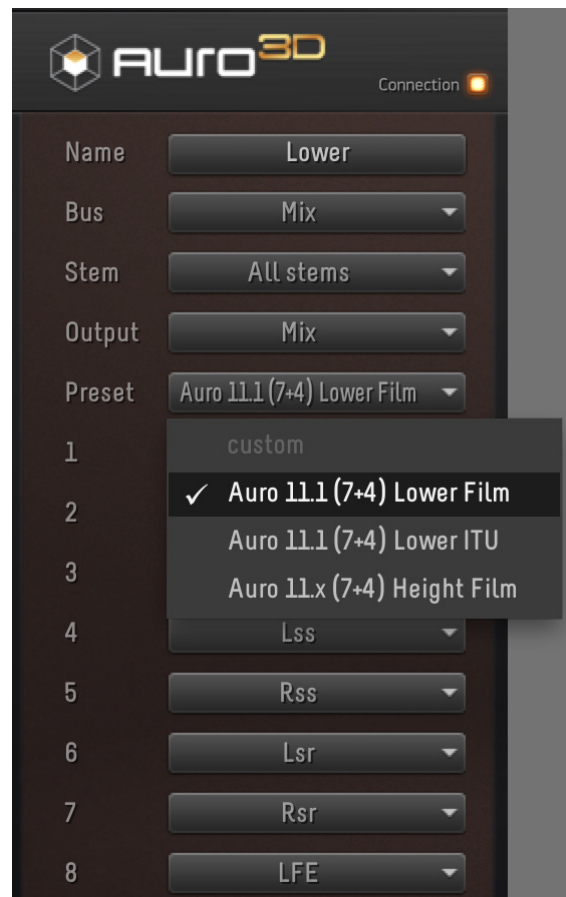
Figure 4-15 Selecting which channels Auro-Return delivers to the DAW
